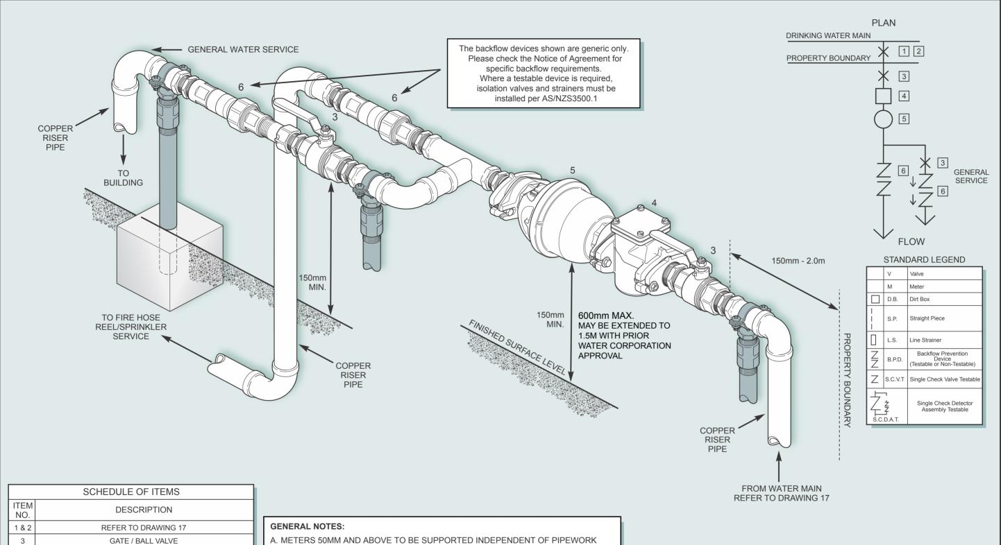
A. METERS 50MM AND ABOVE TO BE SUPPORTED INDEPENDENT OF PIPEWORK
