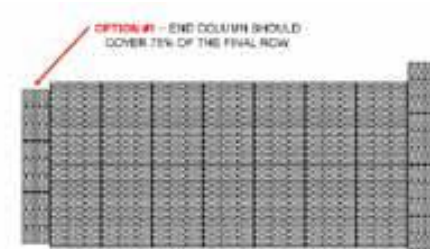
Fig 10: Plan view showing the end row turned perpendicular, corners may not matchup, so 2 options shown.
