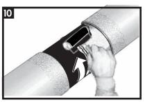
Coat the steel surface and 50mm on to the Sintakote at each side of joint with UCC Protek Butyl Multi Primer.
