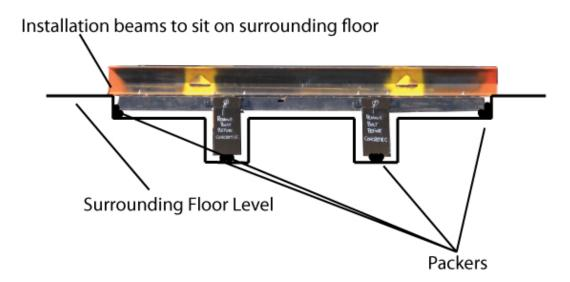
3. Pack under the frame joints, inside the beam rebate and in the corners of the unit to raise the unit 0-2mm higher than surrounding floor level. Packers can be metal, plastic or quickset grout.
