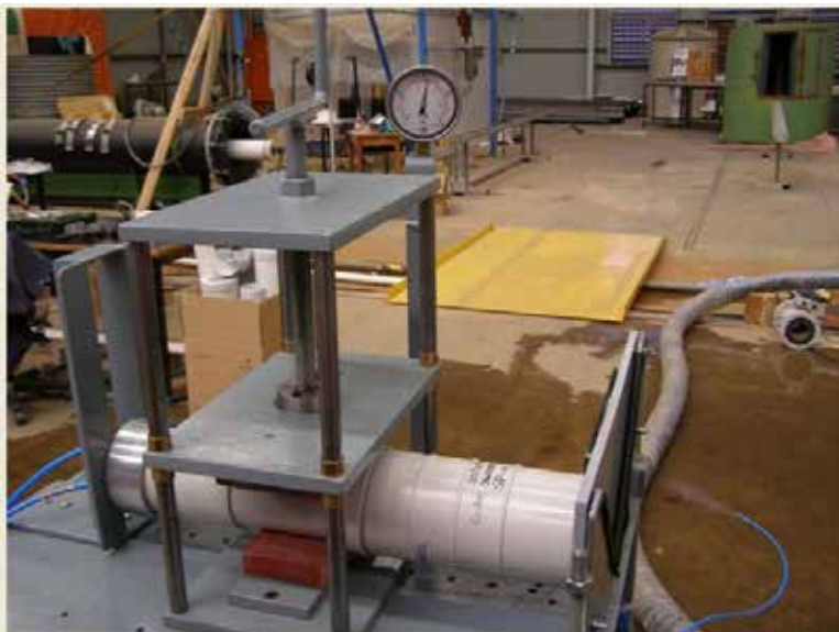
Figure 9: 100mm Expanda Joint DW100150 Hydrostatic test with distortion
