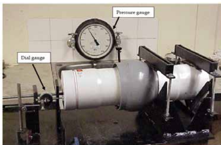
Figure 13: Test rig with swivel joint specimen
