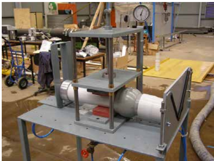
Figure 11: 100mm Swivel Joint SJ10015 Hydrostatic test with distortion
