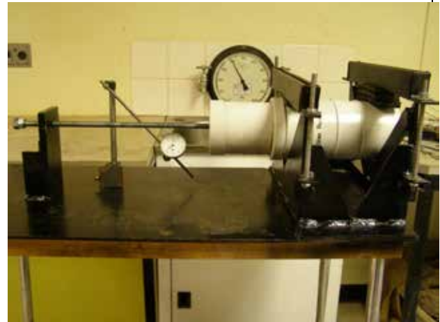
Figure 10: Contact width and pressure on Expanda Joint
