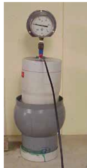
Figure 12: Vacuum test for swivel joint
