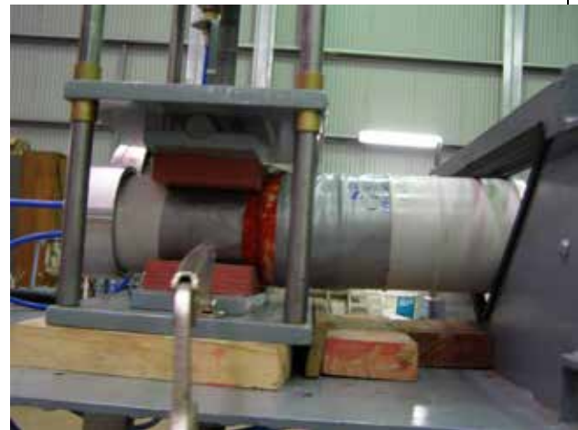
Figure 8: 100mm Expanda Joint DW100150 Vacuum test with distortion
