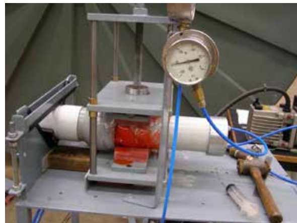
Figure 14: Infiltration test setup showing swivel joint filled with red colour water
